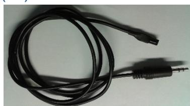
The IR connector detector is used to connect the IR receiver, (shown above). Before connecting the IR receiver make sure the board is switched off. The IR detector must be positioned at the front of your model in a position where it can receive the signal from the remote control handset. Just like your TV remote control if the signal from the remote cannot be seen, the control will not work. The plug on the end of the IR receiver cable is plugged into the IR connector on the board.
