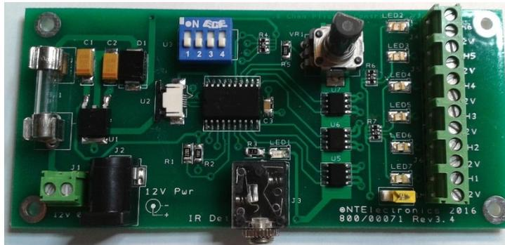
The six-channel flicker unit can control up to 36 off 60 milliamp lights with up to 6 lights per channel. Please refer to the exact capacity ratings [further down this document](#).
