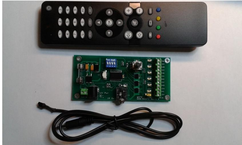
The IR remote control is only used to turn static lights on/off so the option switch 4 must be on for this to work. The IR is not used to control flickering effects.
